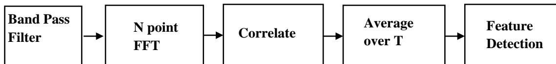
Figure 2: Block diagram of Cyclostationary feature (Shahzad 2010). detection
